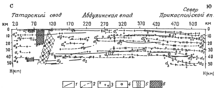
Fig. 1. Comparison of deep crustal sections obtained from refraction deep seismic sounding and "Zemlia" seismologic investigations. (Profile II from Tartar anticline to the North Caspian depression).
