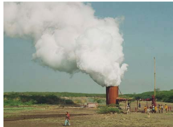
Figure 2: Production test of well TD5 (at well head: T >250 °C, p > 18 bar). The well is located inside the MT survey area.
