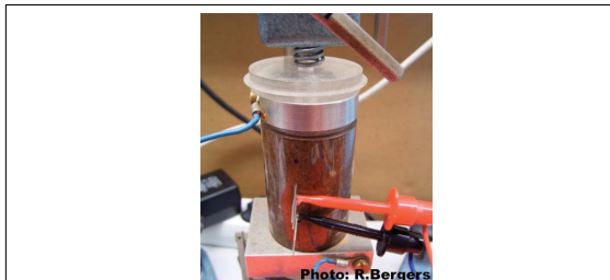
Figure 5: Laboratory geoelectric measuring setup.
