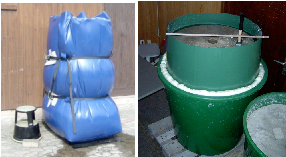
Figure 4: Roman sandstone (left) and Bentheimer sandstone (right). One (left) was wrapped round in a plastic foil, the other (right) was put in a container. Both were saturate with fresh water.
